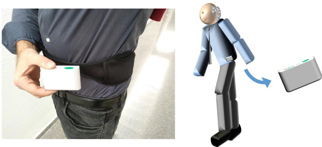
Figure 8. Location and orientation of the sensor
